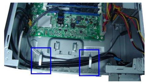
7. Connect the SATA and power cables to their connectors on the rear of the hard disk drive.
